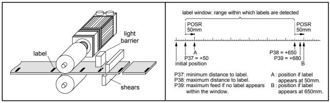
The plate is fed by a roller feed controlled by COMPAX. A reflex light barrier detects the marks on the plate and reports this to COMPAX. The distance between the light barrier and the shears is 50 mm. The shears are controlled and monitored by COMPAX.
